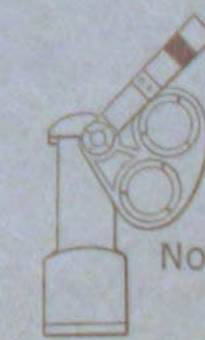
DWARF SIGNAL. Color. YELLOW light at night. Indication. PROCEED with CAUTION. Name. CAUTION Signal.
