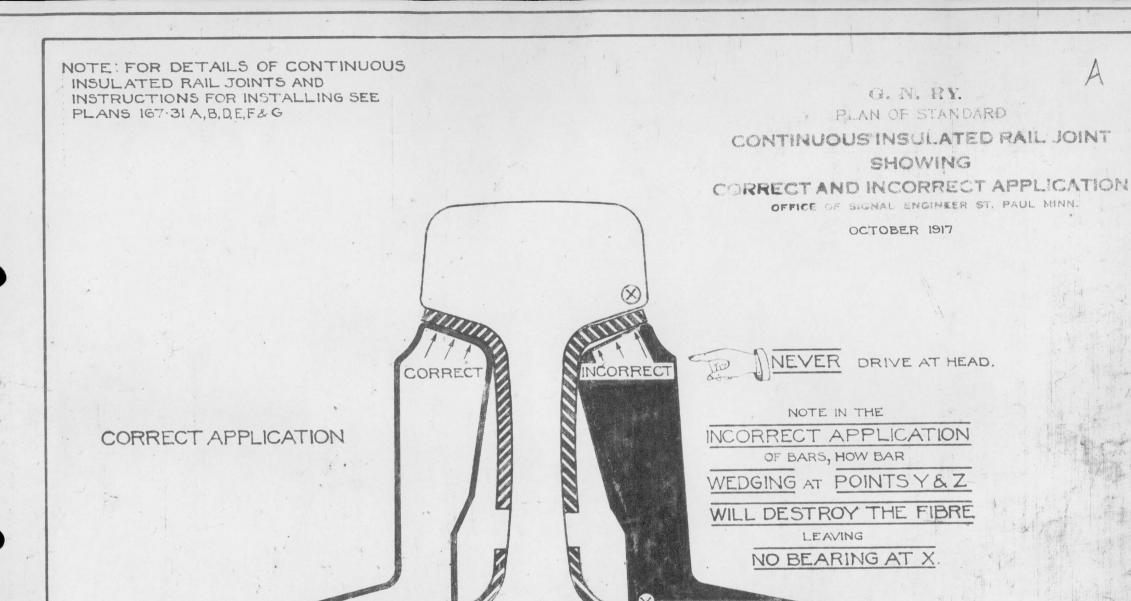
ALWAYS DRIVE AT BASE WHILE TIGHTENING THE BOLTS
