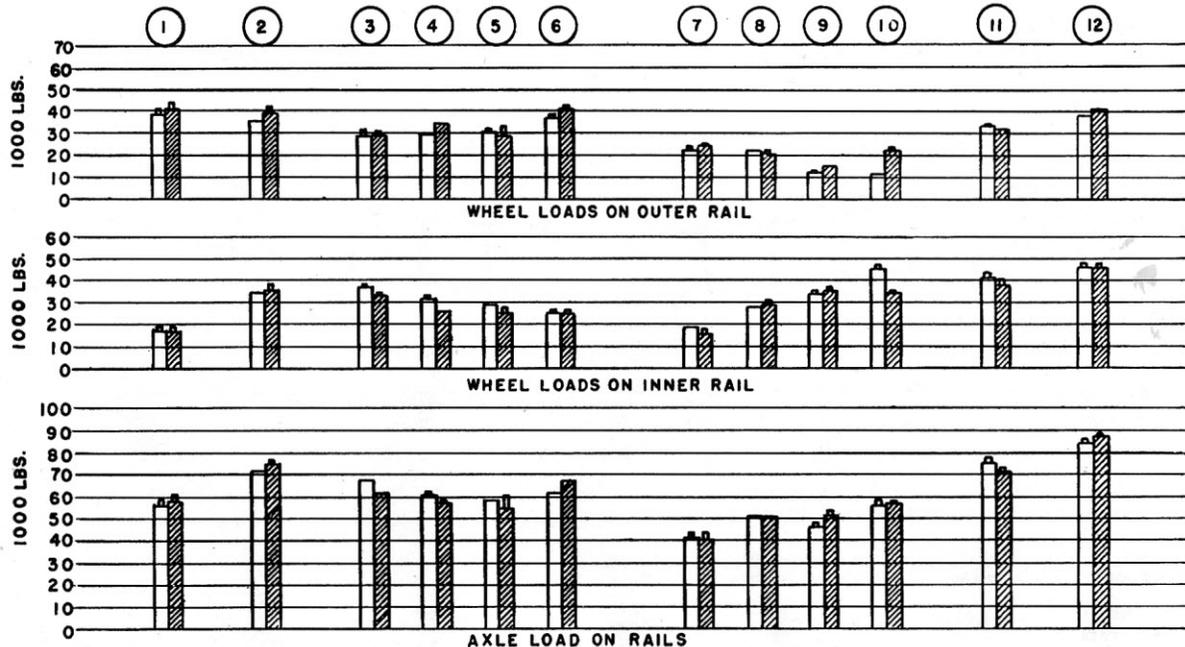
FIG. 5a—VERTICAL WHEEL AND AXLE LOADS DERIVED FROM DIRECT RAIL WEB STRESS ON THE 10-DEG. CURVE AT FOSS RIVER BRIDGE.
