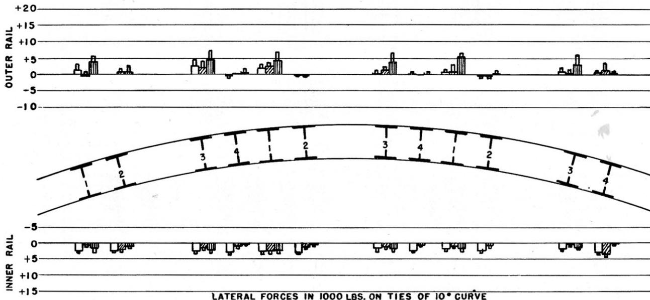
FIG. 10 - MEASURED LATERAL FORCES APPLIED TO THE TIES BY LOCOMOTIVE WHEELS.
