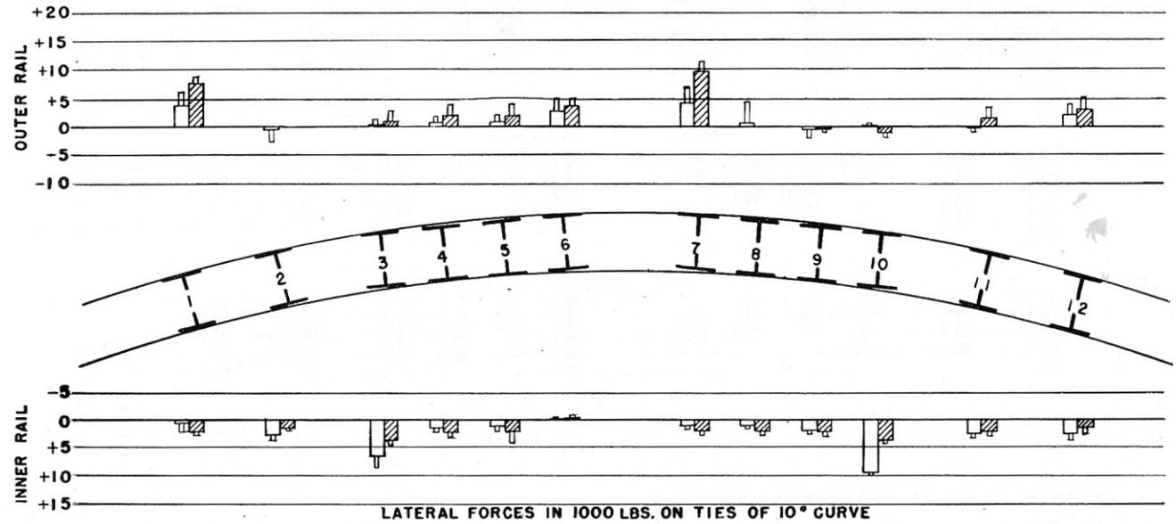
FIG. 5 — MEASURED LATERAL FORCES APPLIED TO THE TIES BY LOCOMOTIVE WHEELS.
