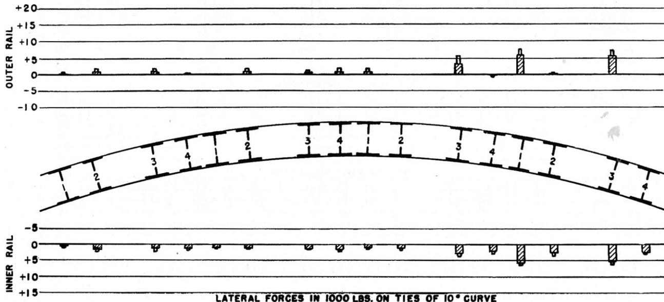
FIG. 20 — MEASURED LATERAL FORCES APPLIED TO THE TIES BY LOCOMOTIVE WHEELS.
