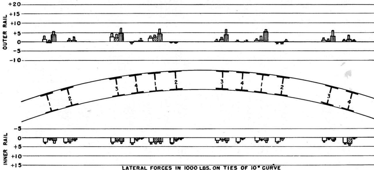
FIG. 10 - MEASURED LATERAL FORCES APPLIED TO THE TIES BY LOCOMOTIVE WHEELS.
