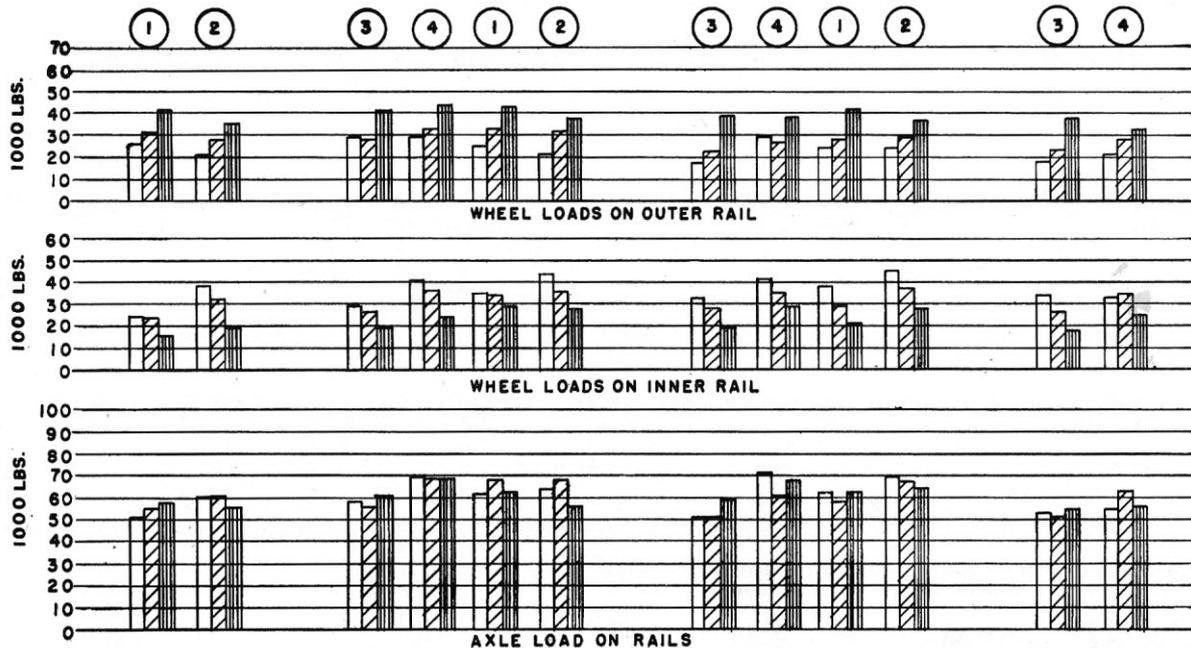
FIG. 10a— VERTICAL WHEEL AND AXLE LOADS DERIVED FROM DIRECT RAIL WEB STRESS ON THE 10-DEG. CURVE AT FOSS RIVER BRIDGE.
