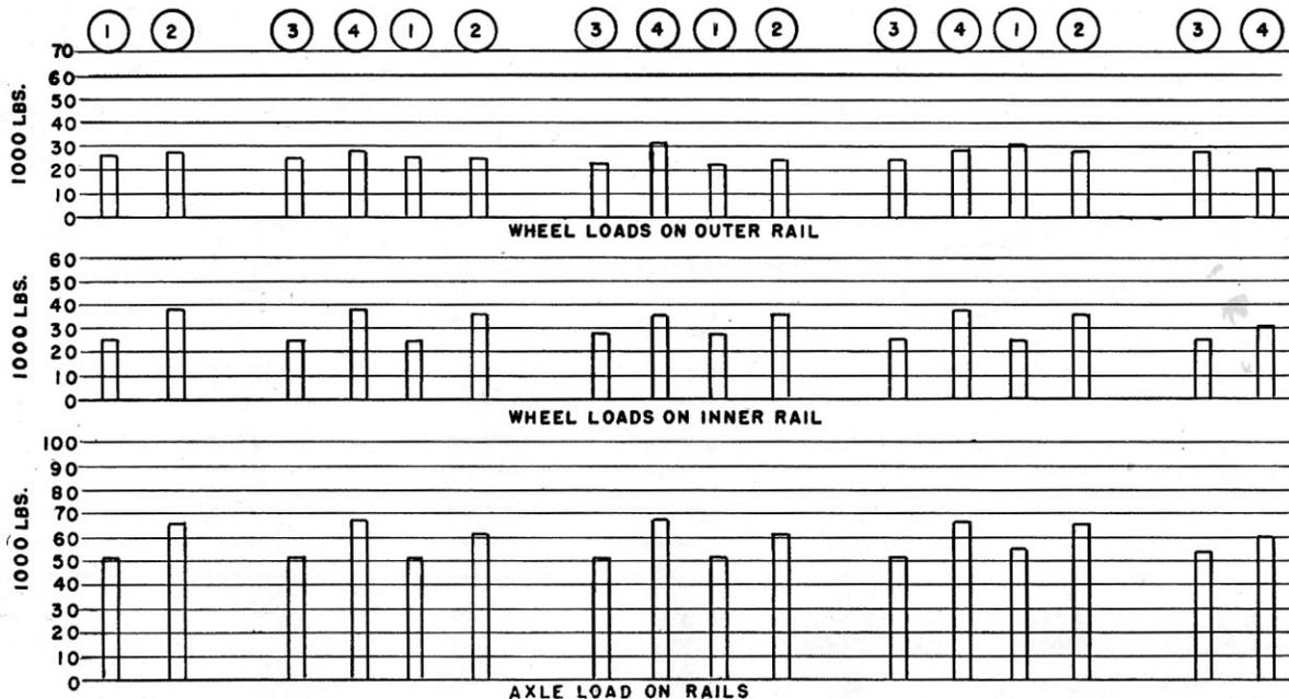
FIG. 20a VERTICAL WHEEL AND AXLE LOADS DERIVED FROM DIRECT RAIL WEB STRESS ON THE 10-DEG. CURVE AT FOSS RIVER BRIDGE.
