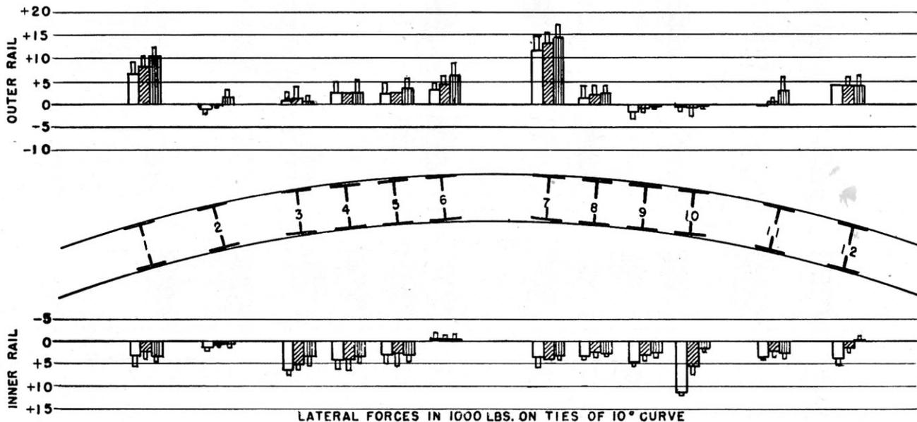
FIG. 1 — MEASURED LATERAL FORCES APPLIED TO THE TIES BY LOCOMOTIVE WHEELS.
