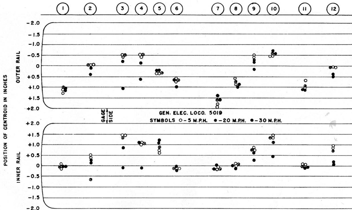
POSITION OF CENTROID OF WHEEL BEARINGS ON 115 LB. RE. RAIL HEADS
