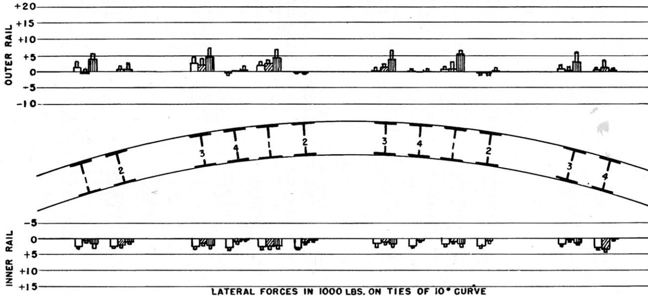
FIG. 10 - MEASURED LATERAL FORCES APPLIED TO THE TIES BY
