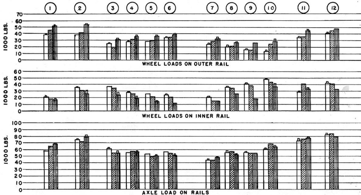
FIG. 1a - VERTICAL WHEEL AND AXLE LOADS DERIVED FROM DIRECT RAIL WEB STRESS ON THE 10-DEG. CURVE AT FOSS RIVER BRIDGE.
