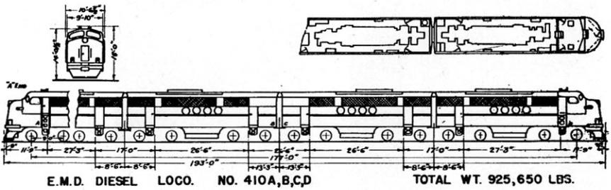
AXLE LOADS & WHEEL SPACING OF LOCOMOTIVES
