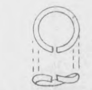
IMP. HI-POWER SPRING WASHER FOR 1" BOLT FIG. J
